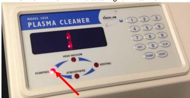
15. When the plasma cleaner is finished pumping the "High VACUUM" LED indicator light will turn on, and a purple plasma light will come on in the window.
