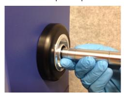
10. Be sure to insert rod with the copper pin aligned with the space in the opening.
