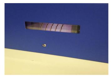
16. The purple plasma light will turn off when the plasma cleaning is complete, once this has happened press vent. The "VENTING" LED indicator light will turn on.
