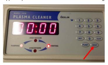
17. Wait 3.5 minutes for machine to fully vent. The machine is fully vented when the "ATMOSPHERE" LED indicator is lit, it is then safe to remove the sample.
