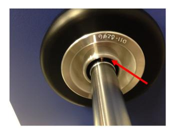
11. Push the rod in until it stops. The photo below shows the rod fully inserted.
